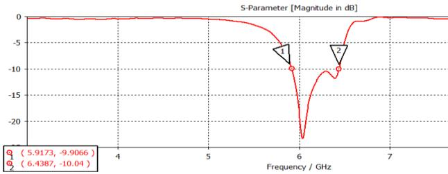
Fig 3. Return Loss ( $S_{11}$ ) of Stacked Antenna Array
