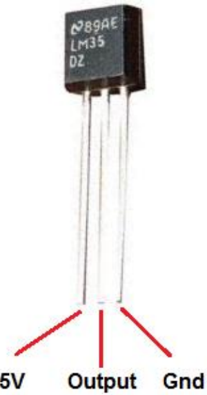
Fig-3: Temperature Sensors
