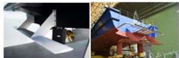
Fig.8. Place Hull Vane in the transom
