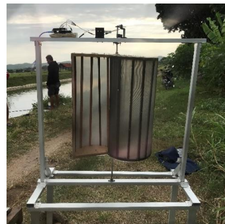
Fig. 11. Implementation of Single-level Savonius Wind Turbine.
