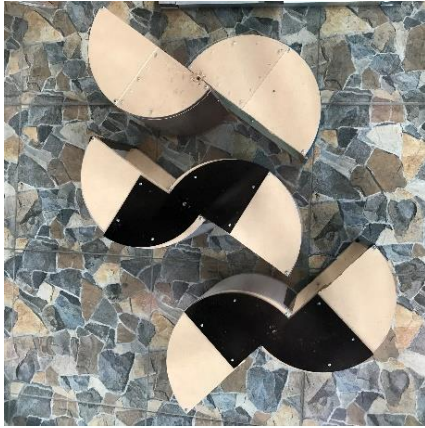
Fig. 12. Multi-level Savonius Wind Turbine with Fixed Rotational Axis Blade
