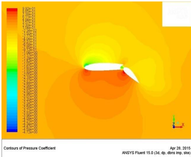
Fig.6. the coefficient of pressure contours on NACA 2412 wing with Single slotted flap at 10°
