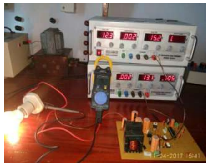
Fig 15. Experimental result showing MPPT operation
