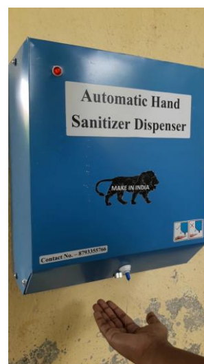
Figure 9. Proposed Automatic hand sanitizer dispenser machine (Wall mounted unit)
