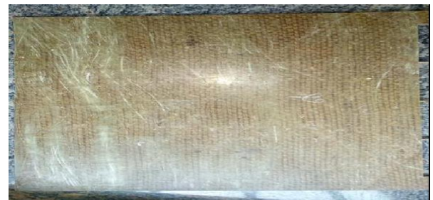
Fig. 2: (a) The sample of Epoxy/S-glass (50%)/jute fiber (10%)
