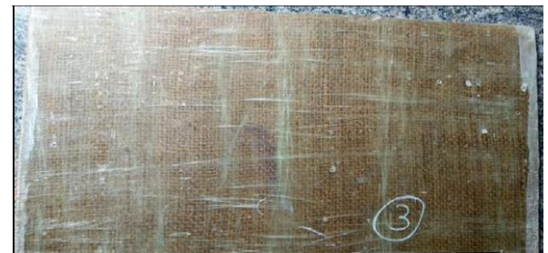
Fig. 2: (b) For jute fiber (25%)
