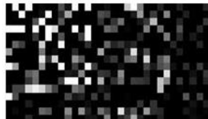
Fig. 4. A sample Hinton map showing the input receptive field of a neuron (from 16x32 Wavelet features) in the trained classifier. The area of each square is proportional to the connection weight it represents, and the color denotes the corresponding sign (red/dark denotes negative, and green/light denotes positive).
