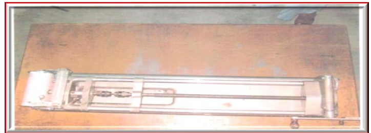
Plate IX: The tensometer used for the tensile test
