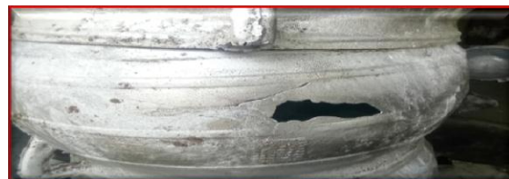
Fig. 2: A pot casting with defect
