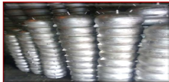
Fig. 1: A pile of visually defects-free pot castings in a foundry shop at Panteka Tudunwada in Kaduna metropolis
