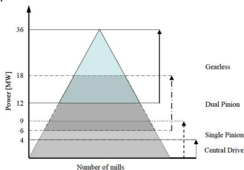
Fig 7.1 Typical mechanical mill configurations [4]
