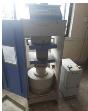
Fig -1 : Testing of Concrete cubes
