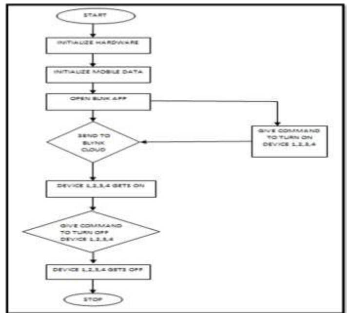
Figure 5: Home automation using BLYNK app
