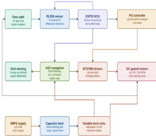
[Fig. 1. Overall system block diagram of the autonomous line-following delivery rover. Insert photograph/diagram upon final submission.]
