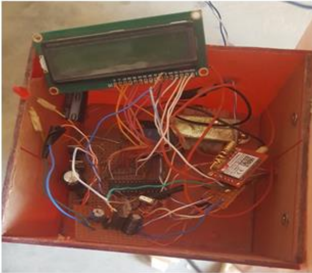
Figure 9. Implementation Garbage Monitoring System
