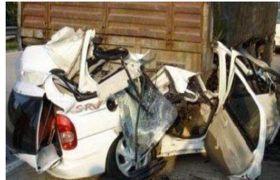
Fig.1 Rear under run collision
