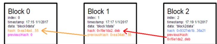
Figure 2. A sample blockchain (with sample blocks)
