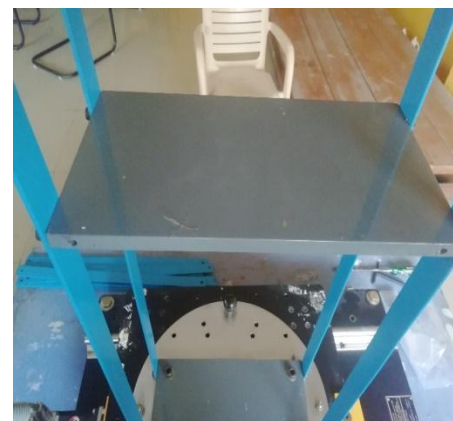
Fig 8: steel plate of thickness 10mm
