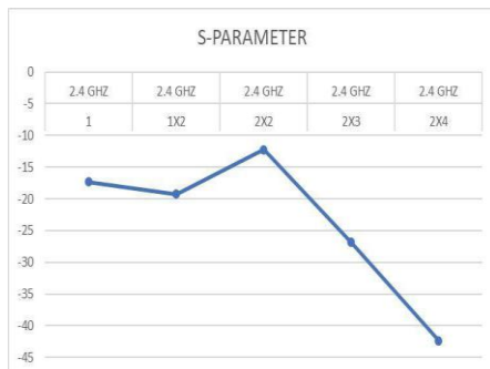
Figure 4.1.1: S-parameter quarter wave feed array antennas
