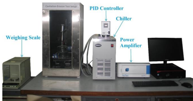
Fig. 2. Vibratory Cavitation erosion Test Setup
