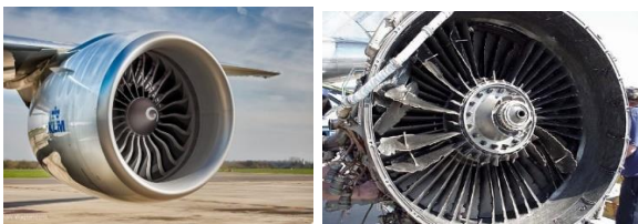
Fig 2. Normal Jet Engine [20] Fig 3. Jet Engine after Bird Strike [21]
