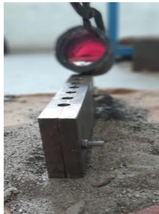
Figure 4. Transfer of cast to mould
