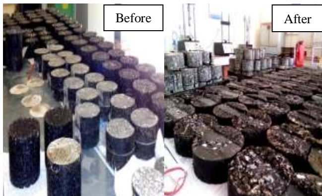
Fig. 10. Gyrotary Samples Before and After Tests
