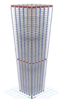
Fig. 5. Model with outriggers at H (top) and H/2
