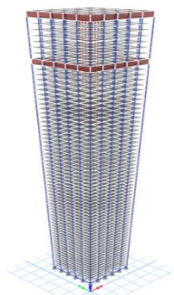
Fig. 2. Model with outriggers at H (top) and 7H/8
