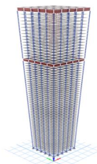
Fig. 3. Model with outriggers at H (top) and 3H/4
