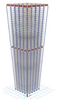
Fig. 4. Model with outriggers at H (top) and 5H/8
