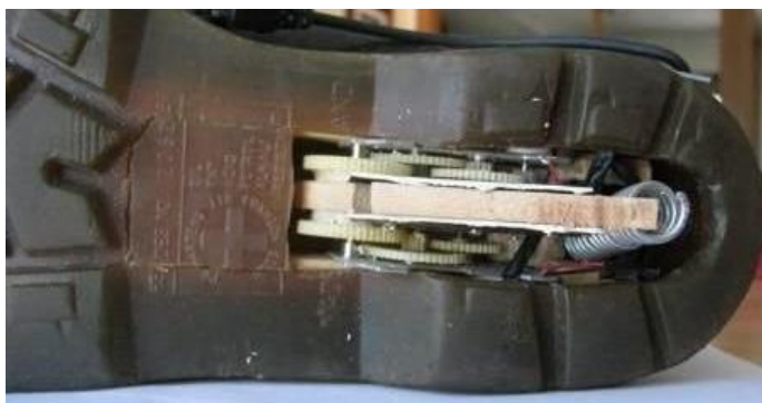
Fig. 3.1.(b) View of arrangement in Power Generation shoe
