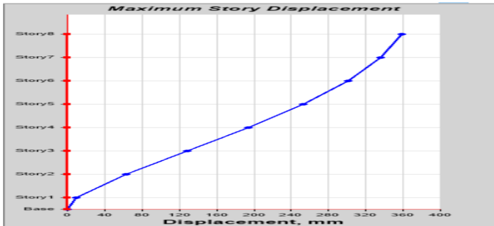
Fig 4.4 Displacement in EQ x direction with SSI for clay soil with X bracing
