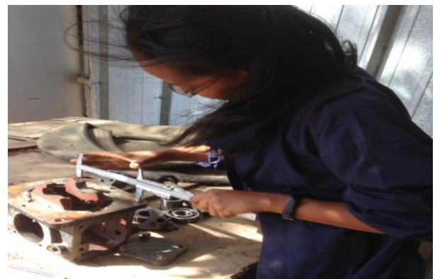
Figure {SEQ Figure \* ARABIC} Manual Technical Measurement of Cherry 100Hp transfer case
