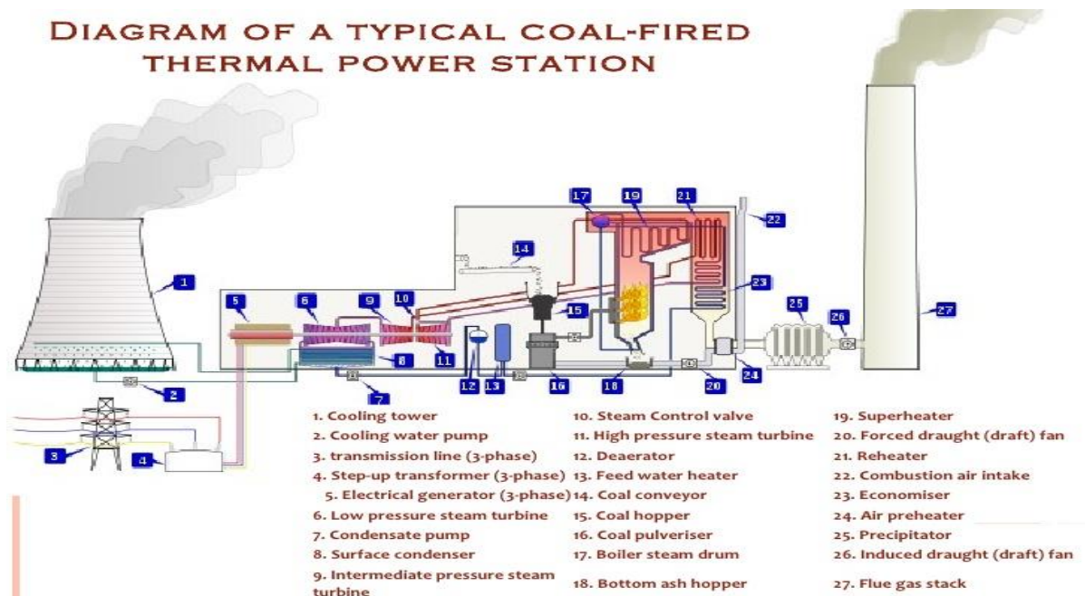
Fig 1 : Typical Coal Fired Power Plant
