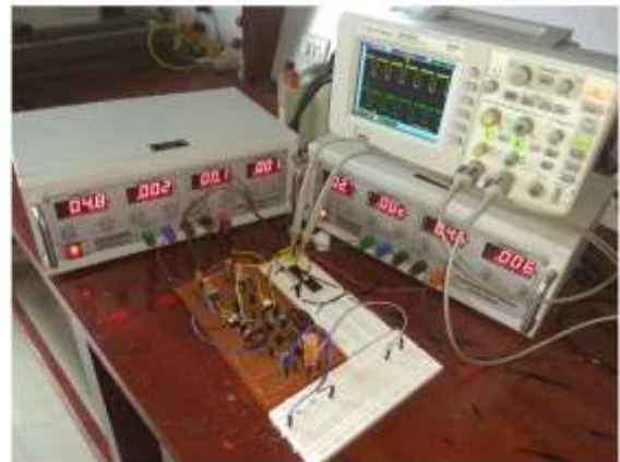
Fig. 13: Experimental setup of Dual Output DC-DC Converter
