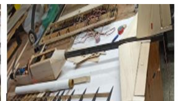
Fig.26 : Fuselage assembly with the tail section
