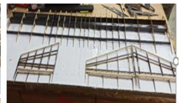
Fig. 24: Horizontal and Vertical tail parts assembly
