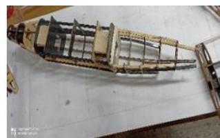
Fig. 25: Fuselage nose section Parts assembly
