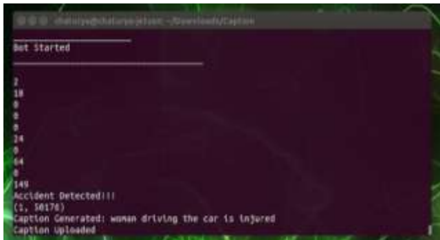
Figure 9 Jetson Nano output after Accident detection
