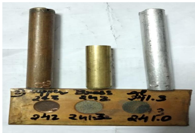
Fig 6. Copper as Specimen and copper, brass, aluminum as electrodes
