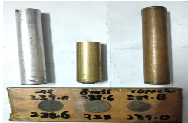
Fig 3. Copper as specimen and copper, brass, aluminum as electrodes
