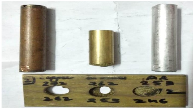
Fig 5. Brass as specimen copper, brass, aluminum as electrodes
