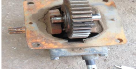
Image 2 Chery 100hp failed transfer case
