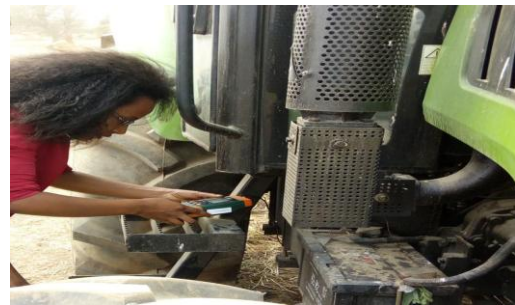
Image 4 the vibration meter magnet tip attachment to transfer case
