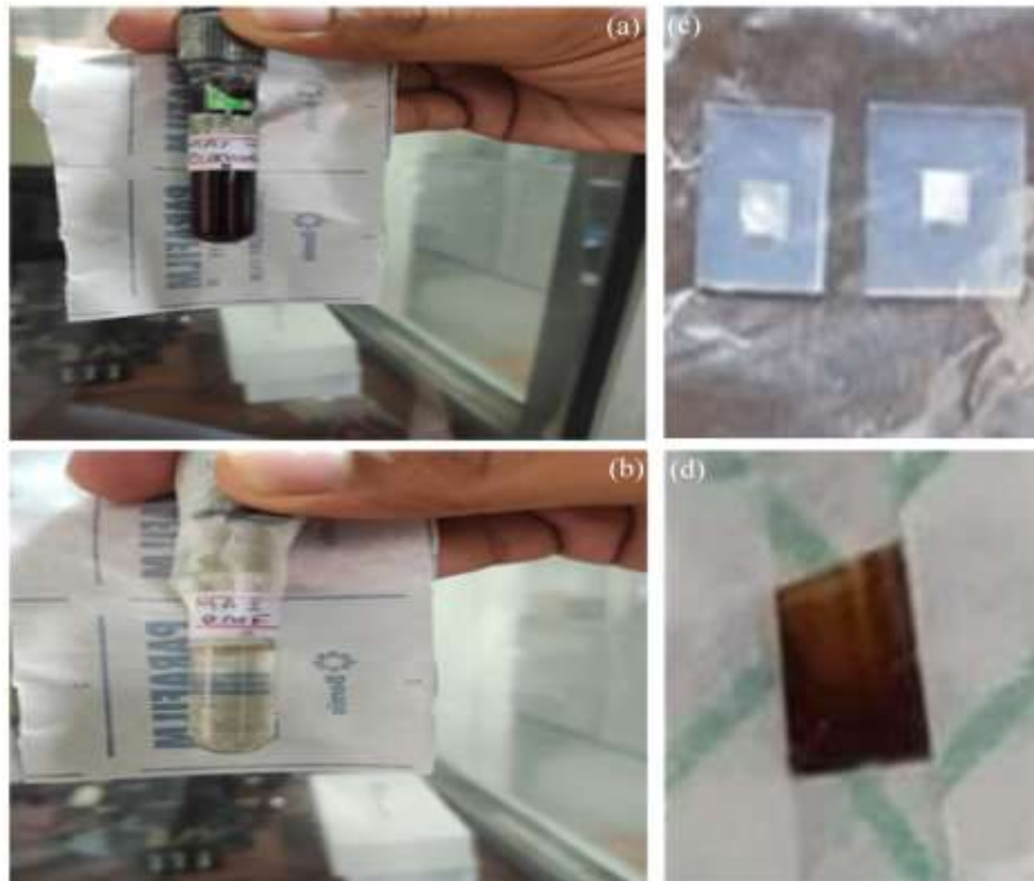
Figure 2:-Photographs of MAI solution in (a) iso-propyl alcohol, and (b) DMF; Photographs of (c) titanium dioxide films, and (d) Perovskite
