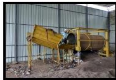
Figure 5: Screening machine used to turn the waste
