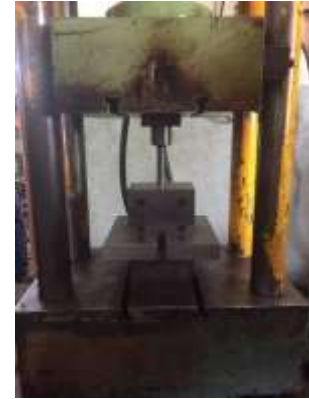
Fig1: Ball milling apparatus Fig 2: Die setup in Hydraulic machine
