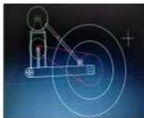
Fig. 6. Chain gear mechanism drawn in CAD
