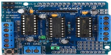
Fig 2.3 - Motor driver L293D
