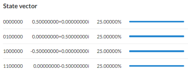
Figure 6. State vectors and probabilities of 4:1:4 Quantum autoencoder with dummy swap gates.
