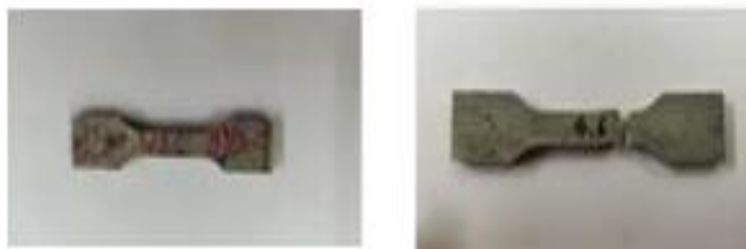
Figure 14 AMC MS-270 specimen-Before and after tensile test
