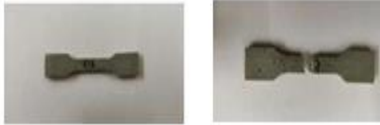
Figure 13 AMC MS-200 specimens-Before and after tensile test
