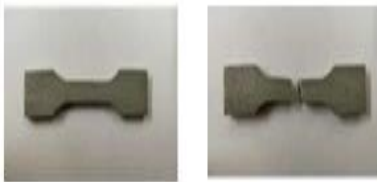
Figure 11 Base alloy specimens-Before and after tensile test
