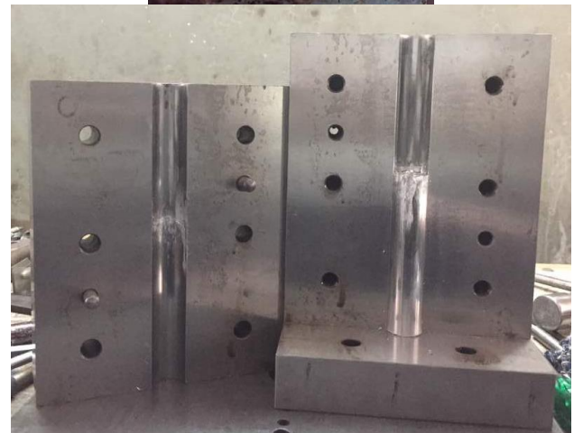
Fig2. Compaction of powder and green compact
