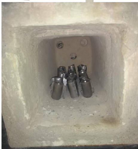
Fig3. Muffle furnace and Sintering of specimens
