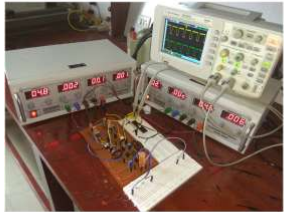
Fig. 13: Experimental setup of Dual Output DC-DC Converter
