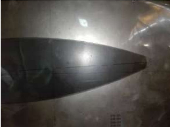
Fig (12) shows the projector bullet photo produced by the imported dies for the quality control department.
