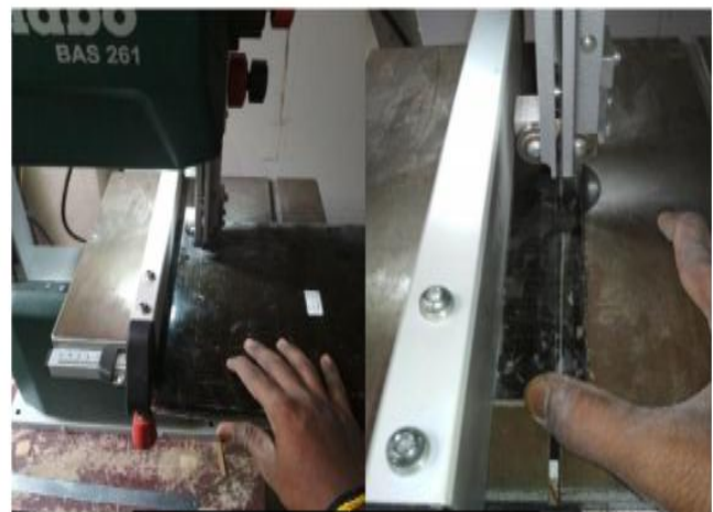
Fig. 4. Specimen preparation using band saw cutting machine
