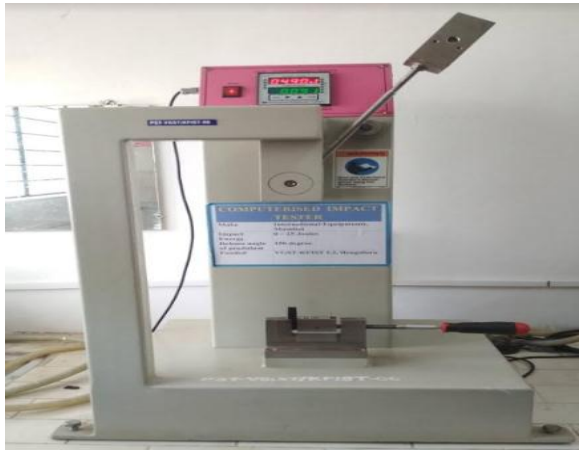
Fig. 5. Computerized impact testing machine
