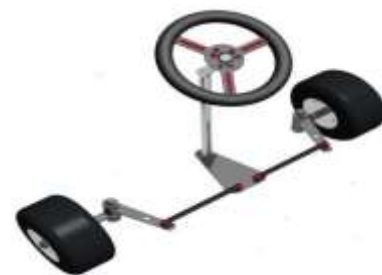
Figure 12: Ackermann steering arrangement
