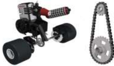
Figure15: Engine coupled at rear axle.
