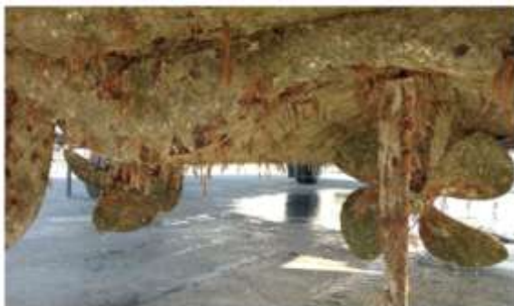
Figure 9 Fouling and Bio Corrosion on the Hull of a Ship
