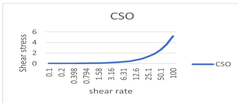
Fig. 10 Shear stress and shear rate graphs of CSO without graphene
