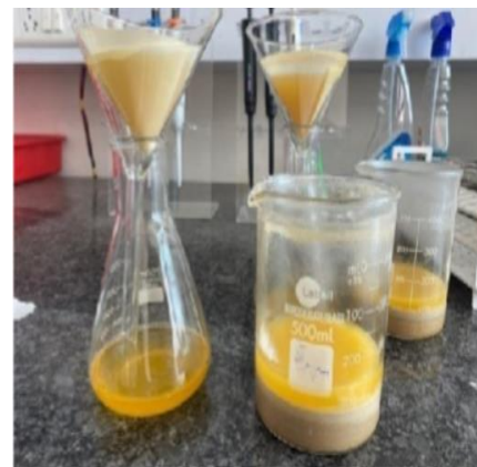
Fig. 9 Oil filtration process
