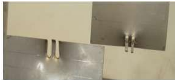
Fig.5 .Pull out failure mode
