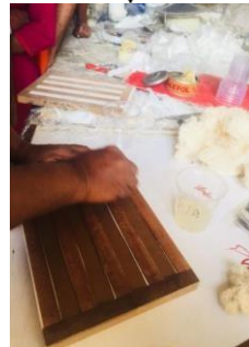
Fig 10: applying PVA coating on mold
