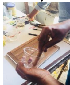
Fig 11: mixing resin and hardener
