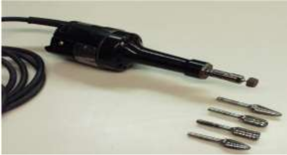
Figure 4: Typical Burr grinder (FHWA, 2013 [6]).
