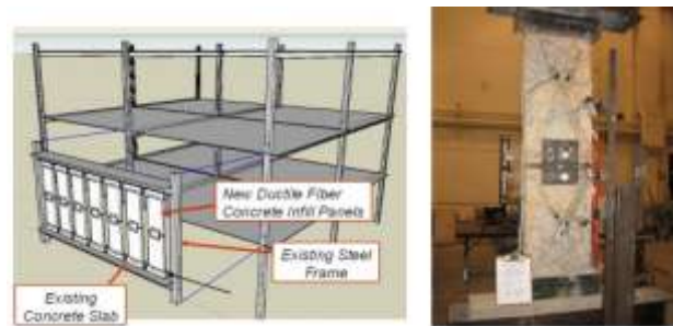
Figure 2. HPFRC infill retrofit system and double infill panel specimen after cyclic testing (Hanson and Billington 2009).
